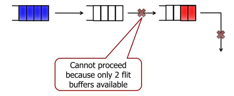
Throughput suffers from inefficient buffer allocation
